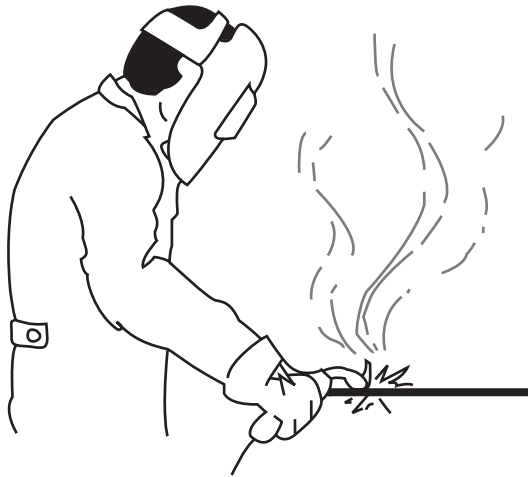
Fig 11. The welder should keep his head outside of the rising plume of air pollutants.
