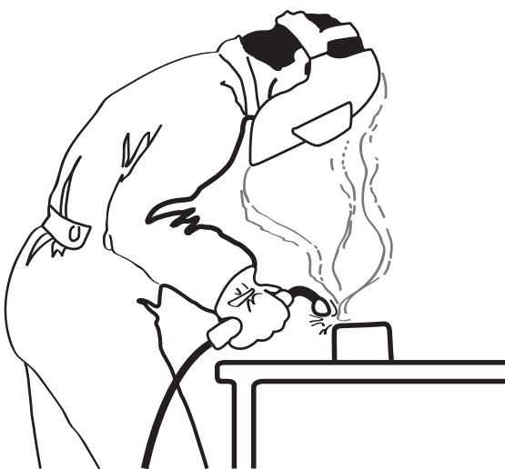
Fig 2. Rising plume of fume and gases from weld spot.
